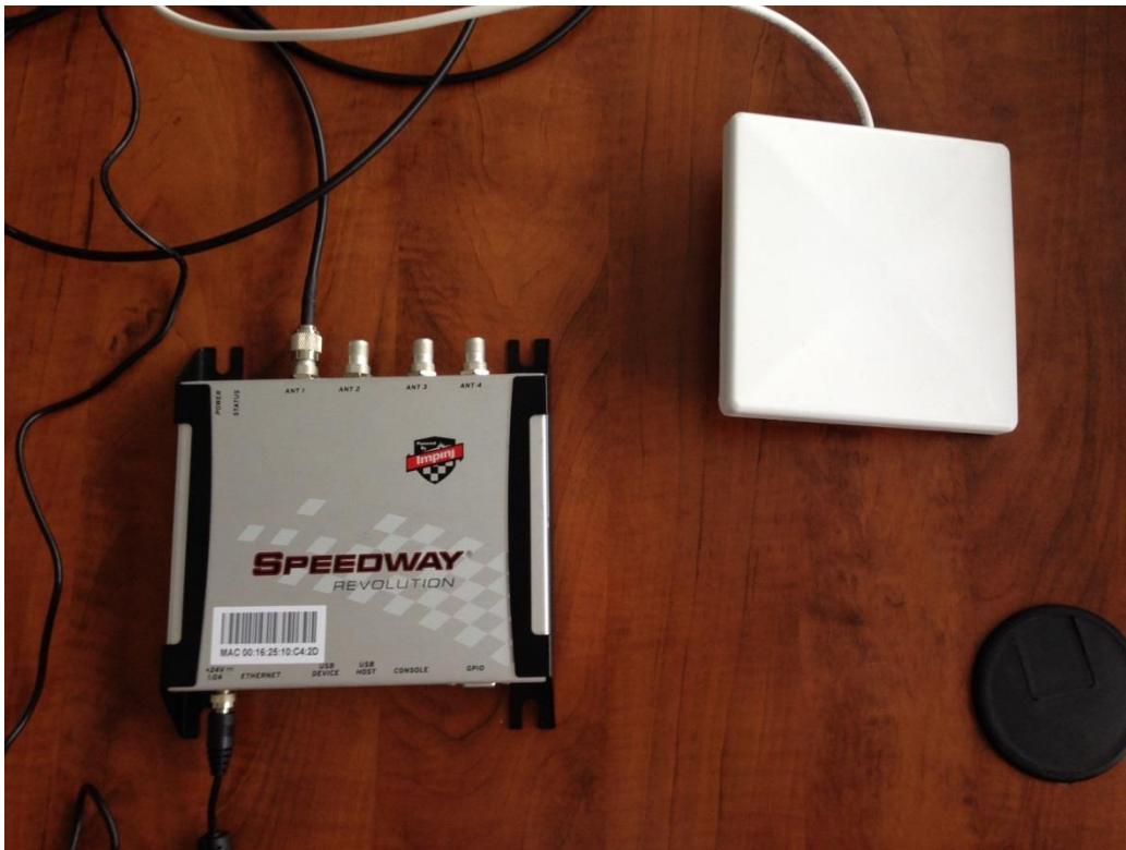
Figure 4: The Speedway Revolution reader with antenna
