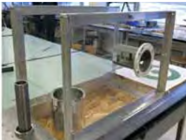
a) Picture of the "Dip Paint & Blow Dry" box through which the cylindrical object will be moving with the help of a device comprised of one or more mechanisms
