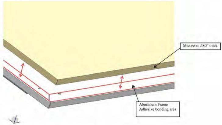
Figure 1. Faces of adhesive bonding (exploded view)
