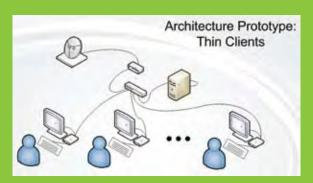
System architecture demonstrating the use of low power dumb terminals passing the workload off to a central server.
