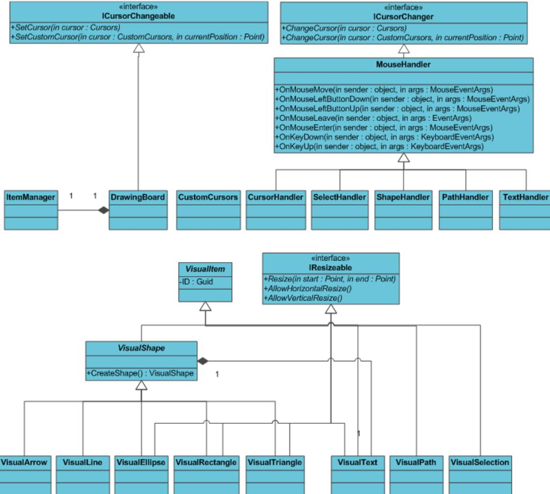
Figure 5: Class Diagram of Classes Supporting User Interaction
