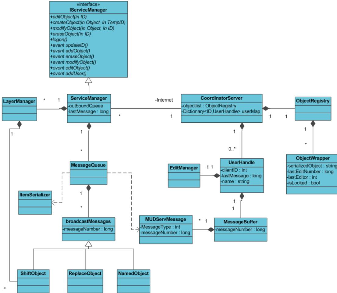
Figure 6: Class Structure of the Server and Related Client Backend
