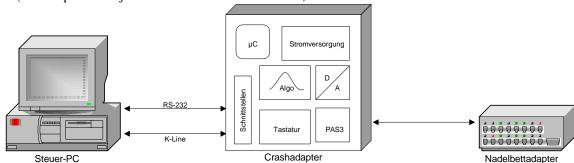
The crash adaptor shall simulate the sensor signals of an airbag ECU to test the crash functions under different conditions.
